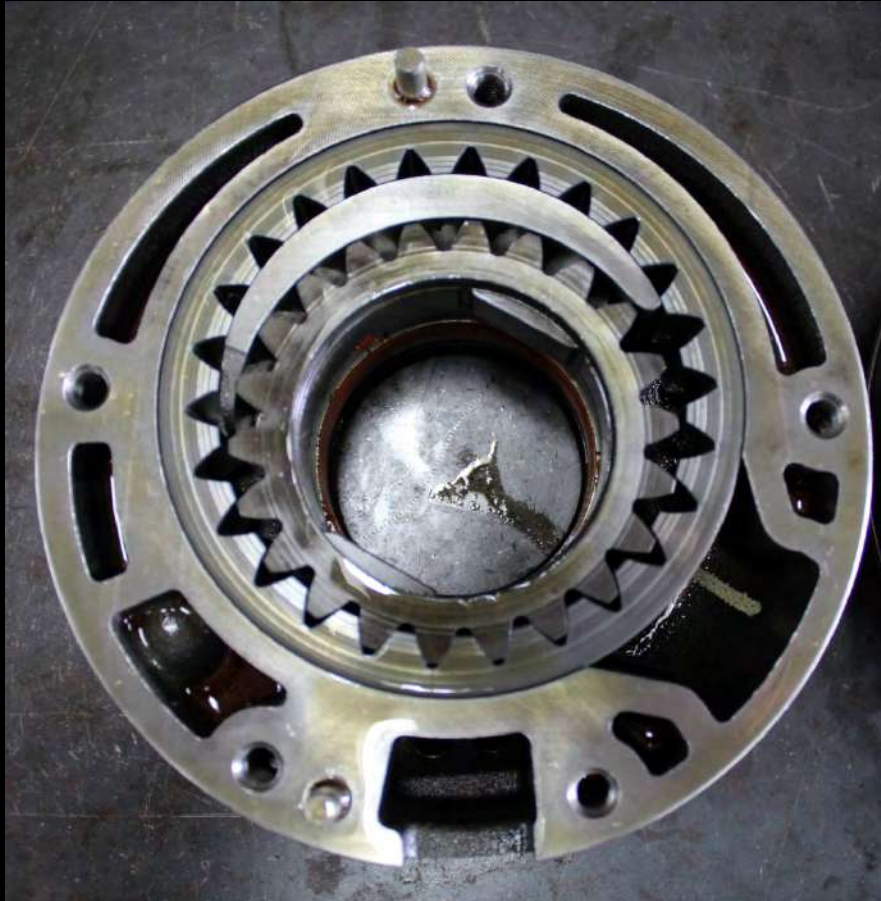
26 TOOTH OUTER GEAR 22 TOOTH INNER GEAR
